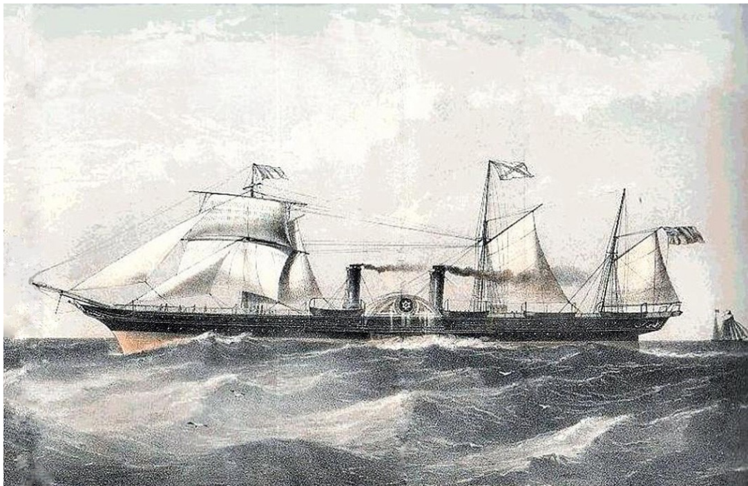
RMS Atrato was originally rigged as a barquentine with auxiliary steam-powered paddle wheels.
